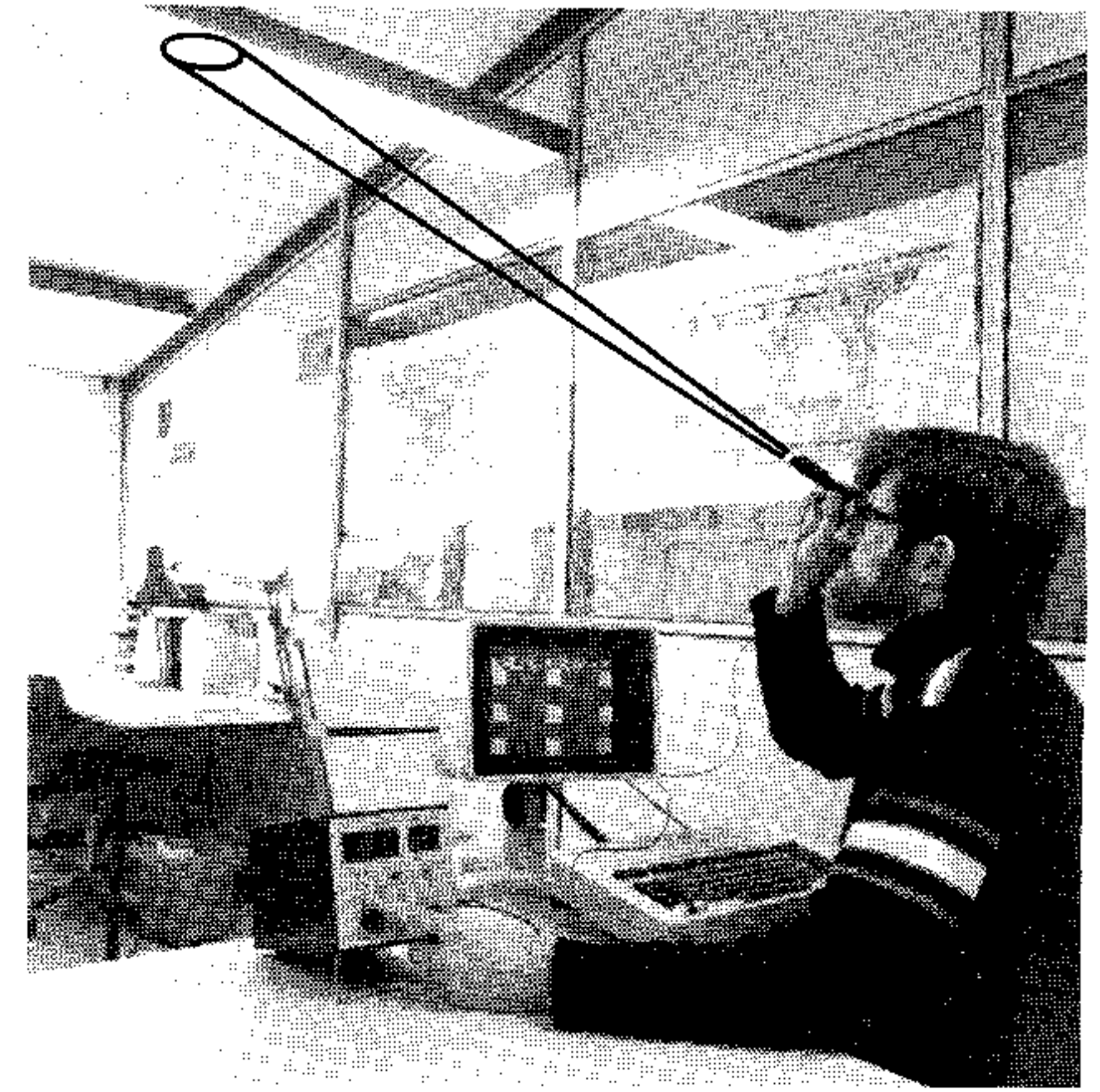
Fig.26. Measurement of the luminance of a luminaire
